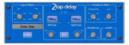
These generate separate left and right delay outputs from a mono'd input feed. Individual tap indicators flash at the current tap rates set. Touch a tap button to highlight it and use the screen encoder to adjust its value, or **tap the button** at the rate you want to set the value.
